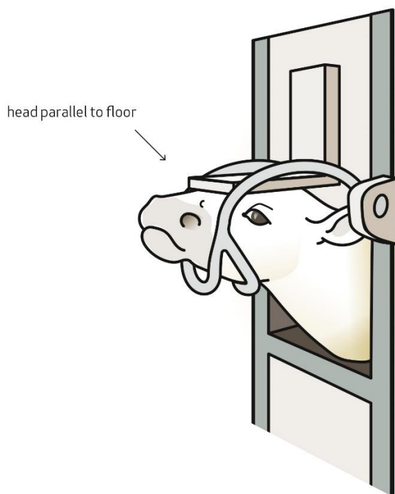
Figure 10. Principle of a neck-yoke for restraining cattle 22
